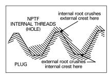
**PTF** fully formed Dryseal threads designed to achieve seal in tapped holes without need for sealing compounds.
